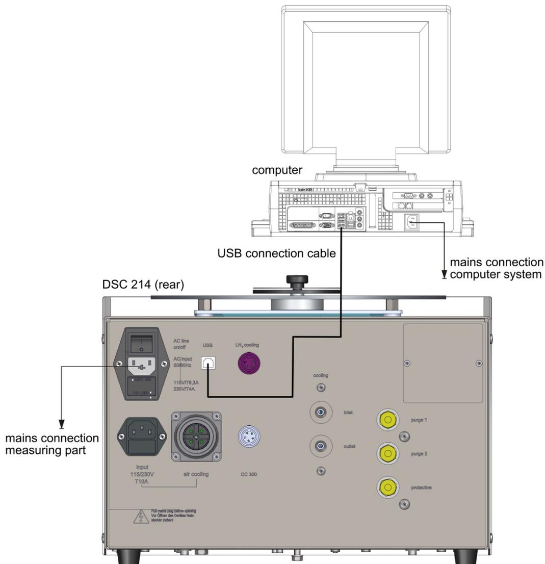
**Figure 1: connecting computer system**
