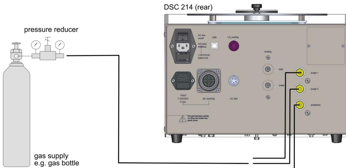
**Figure 12: connecting the gas supply (MFCs)**
