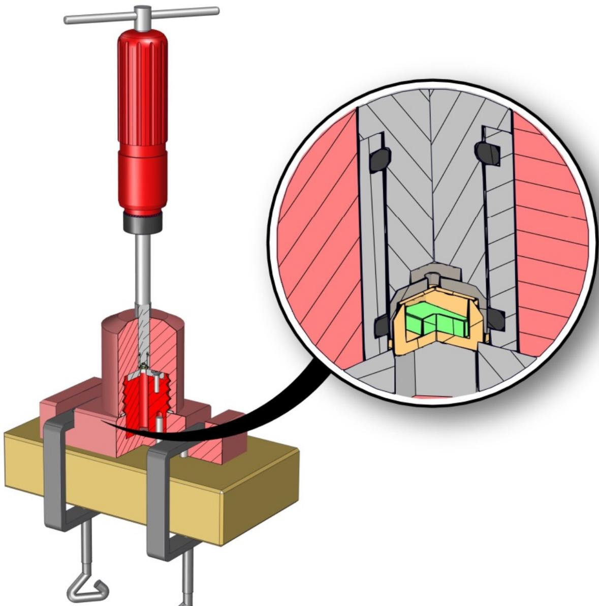
**Mounting the Support Fixture for High-Pressure Crucibles**
