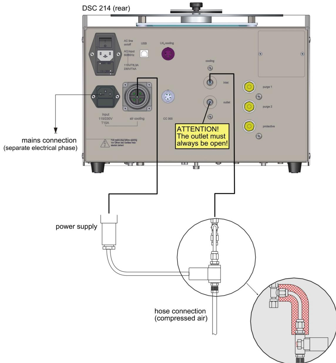
**Figure 3: connecting the on-off valve kit for compressed air cooling**
