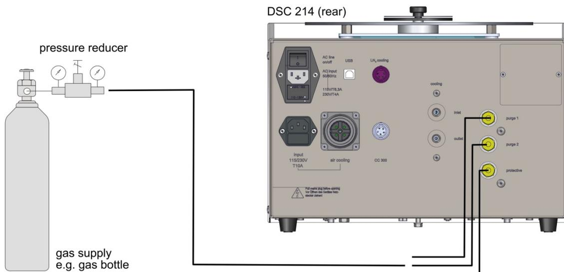
**Figure 10: connecting the gas supply (sintering inserts)**
