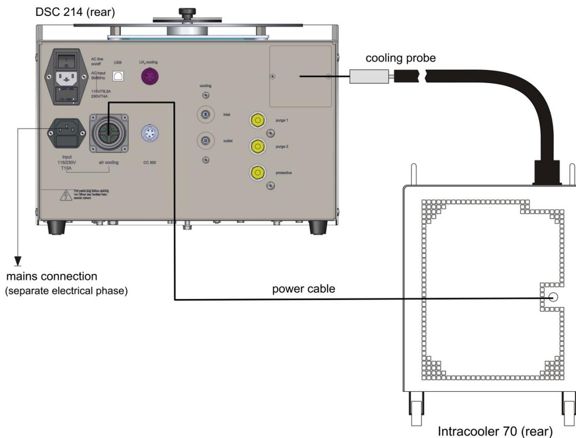
**Figure 6: connecting the Intracooler 70 (230 V / 50-60 Hz)**
