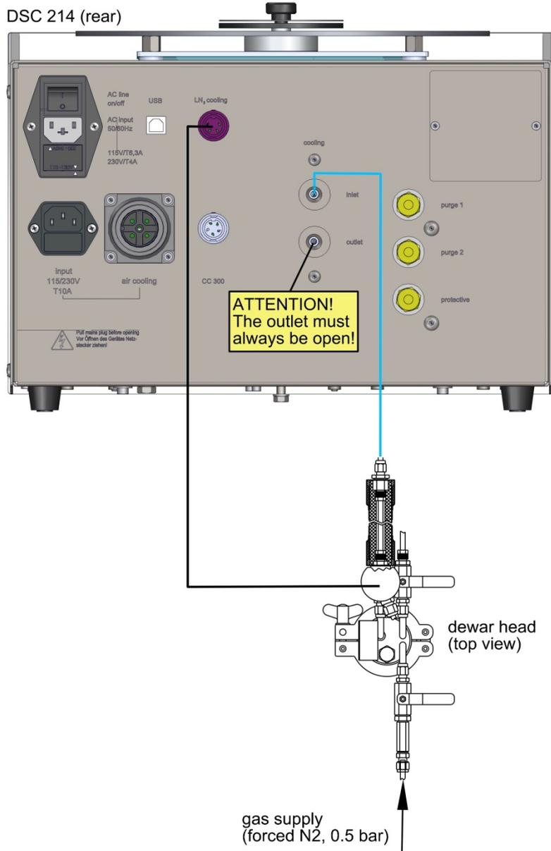
**Figure 8: connecting the LN2 cooler CC 200 F3 with magnetic valve**
