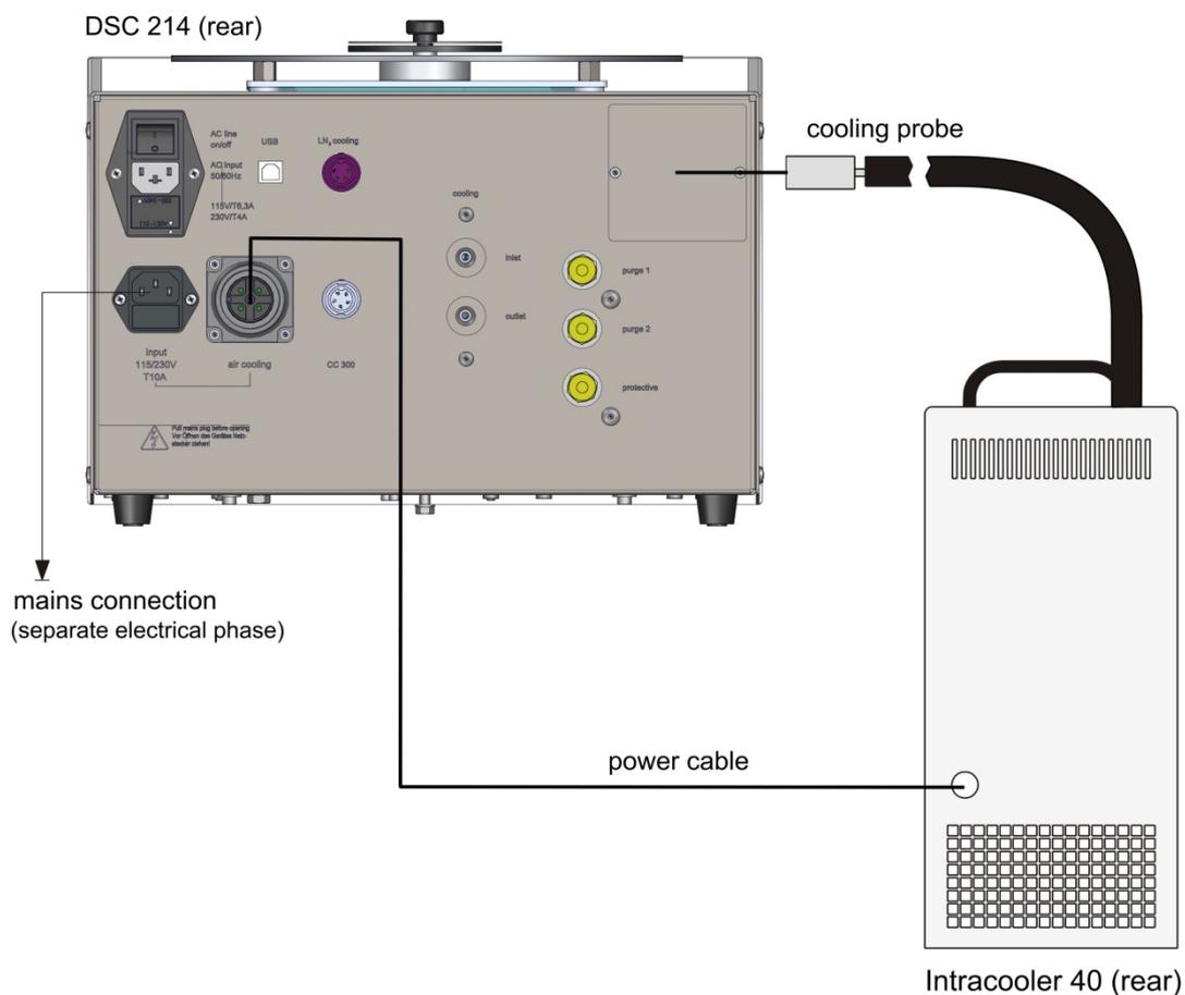
**Figure 5: connecting the Intracooler 40**
