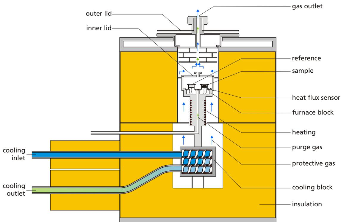
Figure 13: DSC 214 cross-section of the measuring cell
