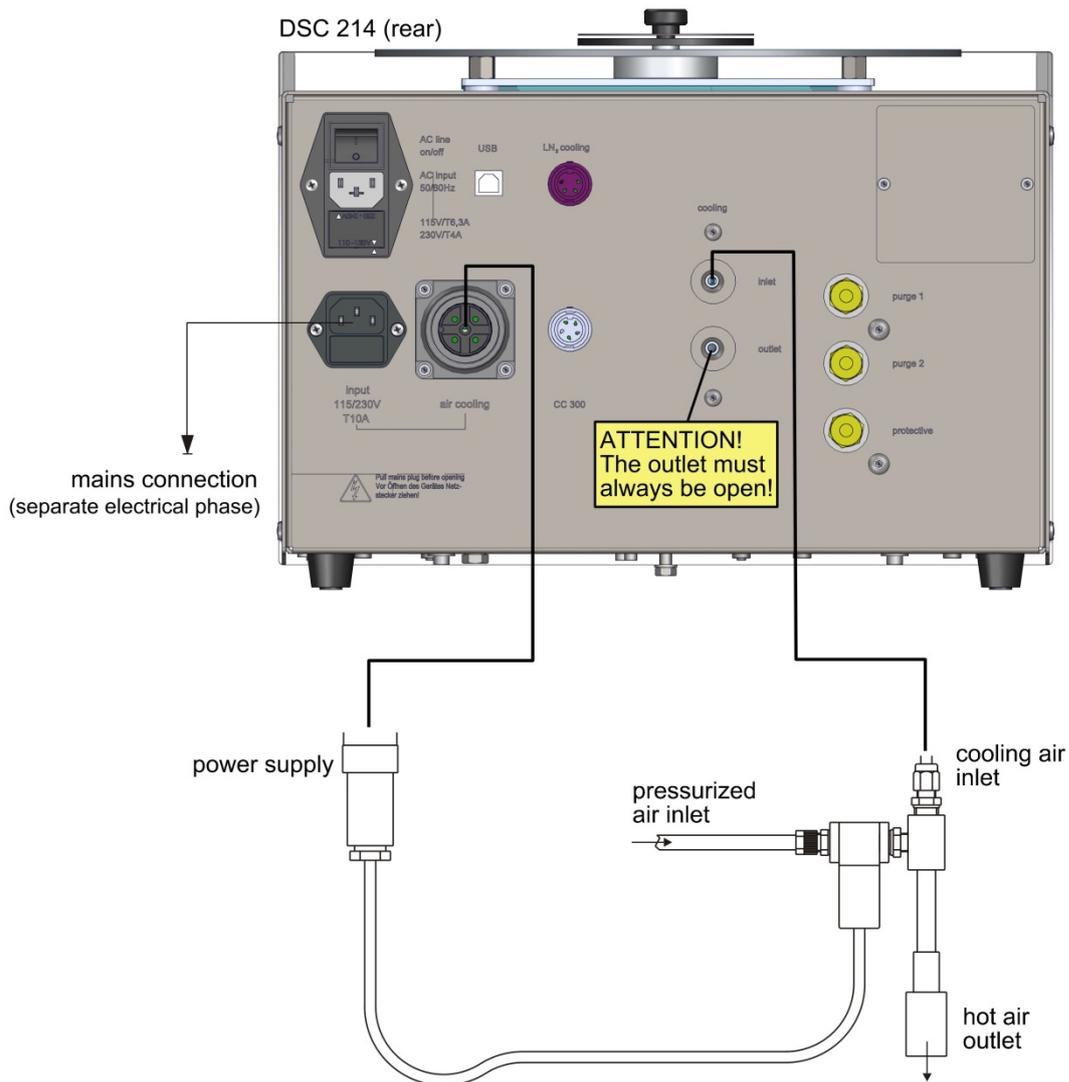
Figure 4: connecting the cooling device for pressurized air
