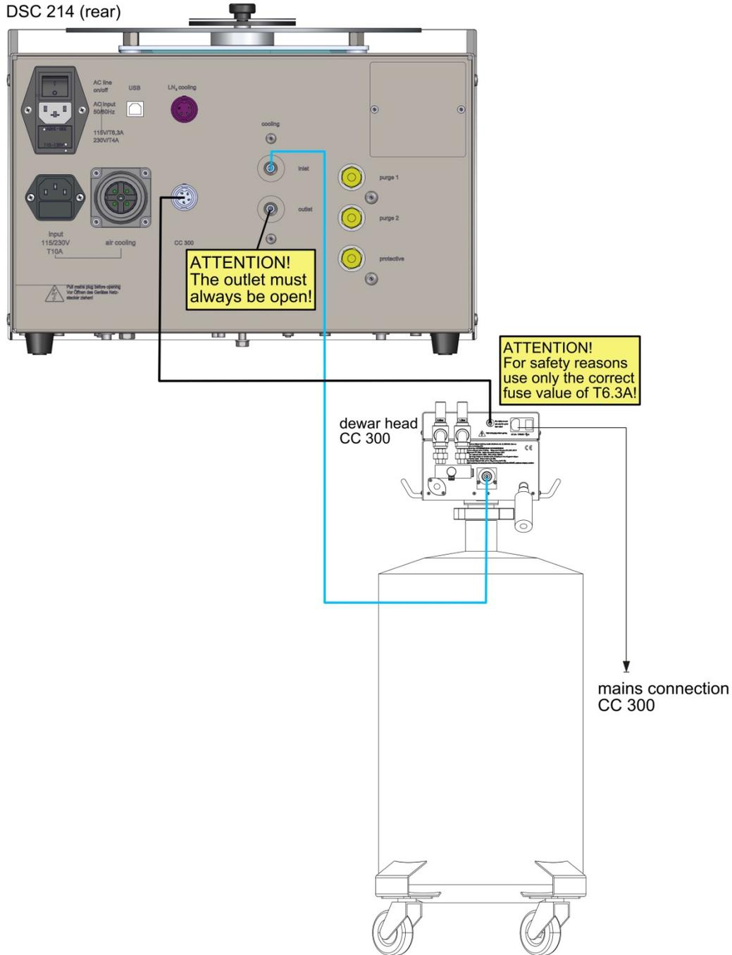
**Figure 9: connecting the LN2 cooler CC 300**
