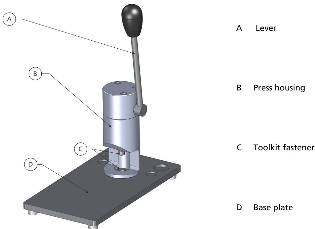
Sealing press no. 6.240.10-80.0.00 is used for sealing different types of crucibles. Each type of crucible requires a different toolkit (see available toolkits). To seal a crucible, position it on the lower part of the toolkit fastener along with its corresponding lid. Then lower the lever with a single continuous motion to close or cold weld the crucible. The necessary force is defined by a spring in the press housing.
