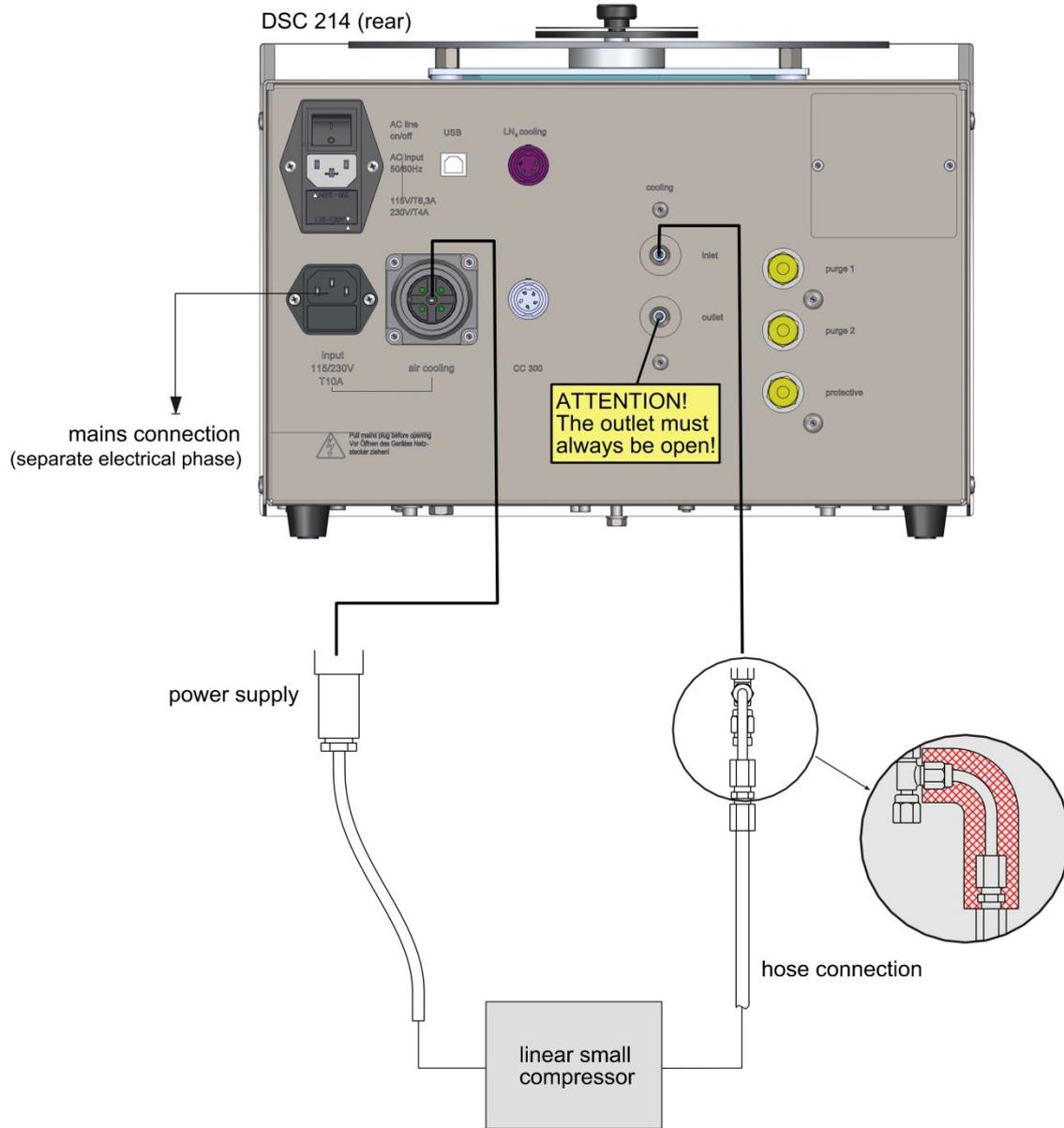
**Figure 2: connecting the linear small compressor**
