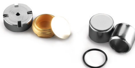
Medium-pressure crucible (right) and high-pressure crucible (left)
