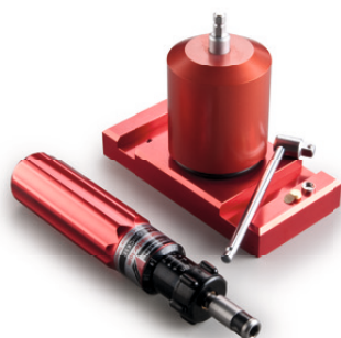
Sealing tool for the high-pressure crucibles, order no. 6.239.2-92.4.00
