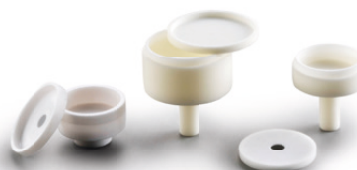
Crucibles for TGA Sample Carrier (HTP40000A52.000-00) of the STA 449 F1/F3 Jupiter®
