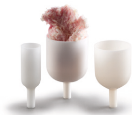
Al 2 O 3 crucibles with different volumes (0.9 ml, 3.4 ml, 5 ml)
